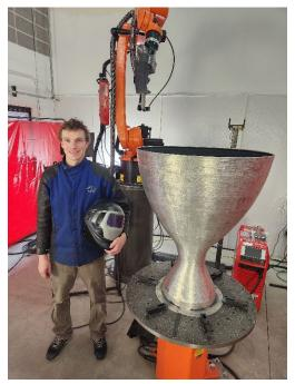
Fortius Metals is launching our first advanced welding alloy, A6061-RAM2, which solves the traditional problem of hot cracking and hot tearing. Fortius 6061 welding wire also show tensile strength above typical values for wrought, using the standard T6 heat treatment. Our welding wire can be used for traditional welding and joining, and is a great candidate for large format metal 3D printing like WAAM and laser wire DED.
